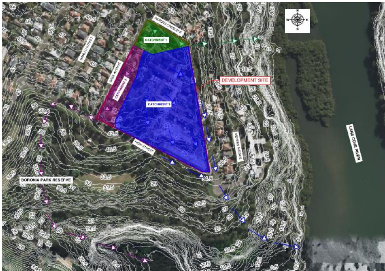
Figure 2 Existing stormwater sub- catchments
